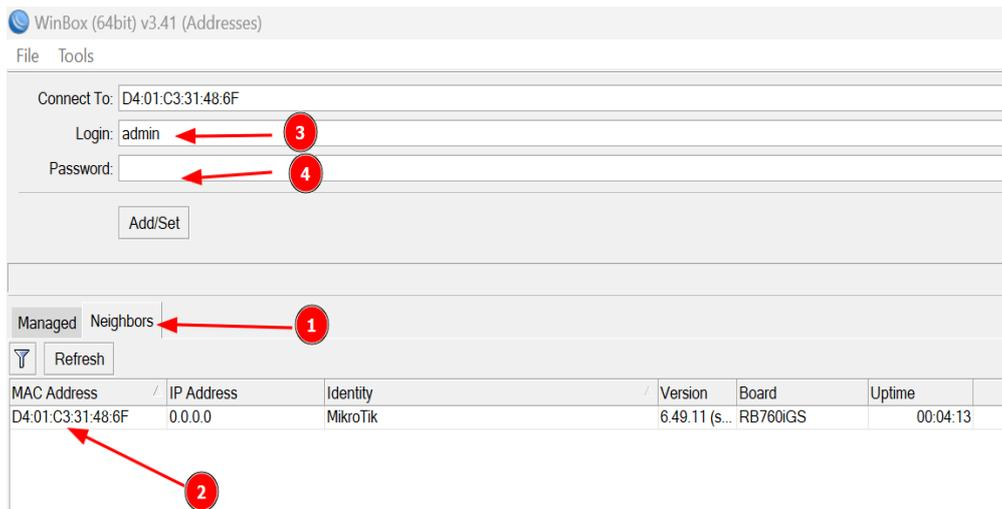
Login to the Mikrotik BDR with the password at the back of the router
